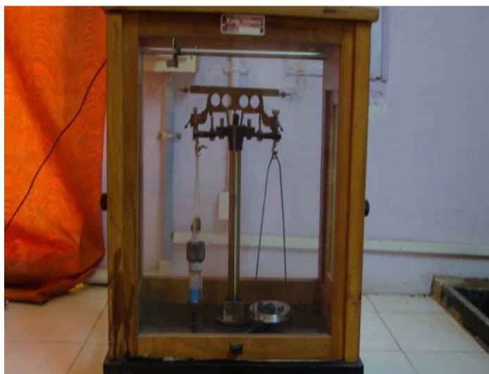
Figure 1: Modified physical balance for buccoadhesive strength measurement
